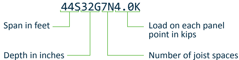
Figure 284: STAAD.Pro nomenclature for SJI joist girders
